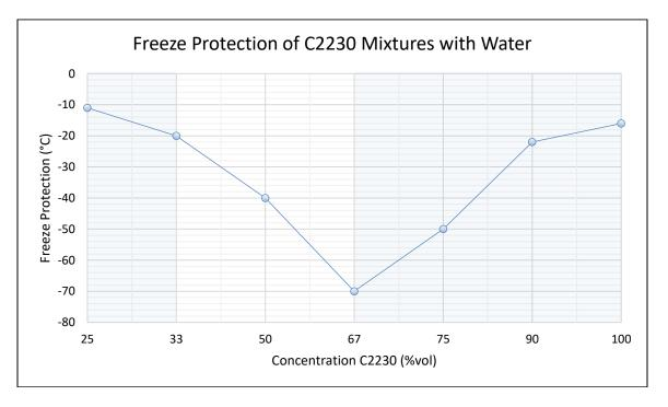
Freezing Protection = Average of Freezing Point (ASTM D1177) and Pour Point (ASTM D97)
